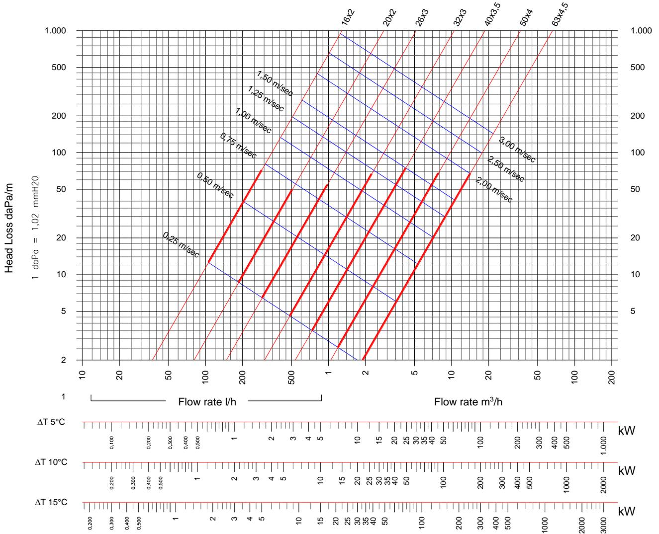
The graph shows the pressure drop as a function of the fluid flow rate in l/h or in m<sup>3</sup>/h or as a function of the system potential in kW (please use the scale suitable for the  $\Delta T$  temperature gradient of the water).
