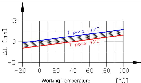
The diagram on the side shows the linear expansion of 1 m of pipe (measured at a "T<sub>Laying</sub>") as soon as the pipe is put into operation.
