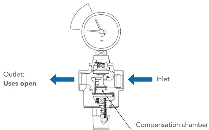
When the uses are opened downstream, the pressure exerted on the piston is lessened in favour of the force exerted by the spring on the shutter permitting it to open with the constant passage of the fluid. As the water demand from the user network increases the pressure on the piston decreases and more water passes.
