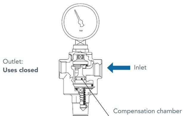
When the uses to be served are closed, the downstream pressure increases, pushing the reducer piston downwards. In this way, the shutter closes the passage section of the reducer maintaining the setting value set on the spring constant; in fact, the minimum pressure difference across the shutter permits the perfect closing of this latter.
