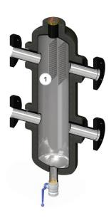
1 Double cloison Brise flux
